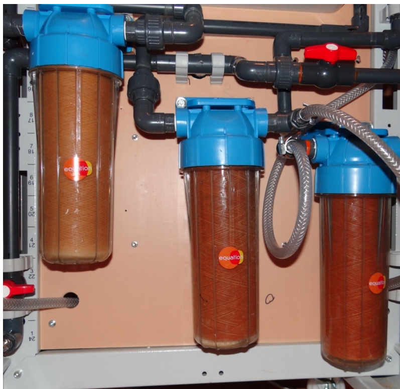
Fig. 6. Appearance of ten micron filters of the experimental EMERALD-UNIVERSAL-500 device after 4 hours of operation on fresh artesian water with the content of ferrous ions about 4 mg / l.
