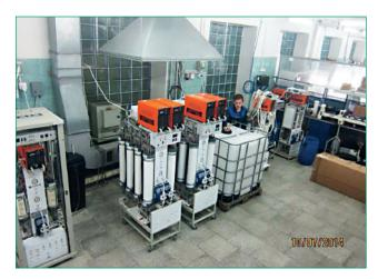
**Fig. 6.1.2.** AQUACHLOR-1500M devices with a chlorine capacity of 1.5 kg per hour with MB-26D modular electrochemical elements in a dielectric body. The AQUACHLOR-1500M device contains 8 MB-26 elements of model 28600M1P4–05. Electric power consumption is 7.0 kW, weight 600 kg.
