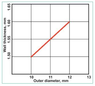
Fig. 6.1.7. Size ratio of ceramic diaphragms for MB-11 elements.
