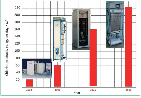
Fig. 6.1.10. Productivity of AQUACHLOR devices referred to the floor area they occupy.
