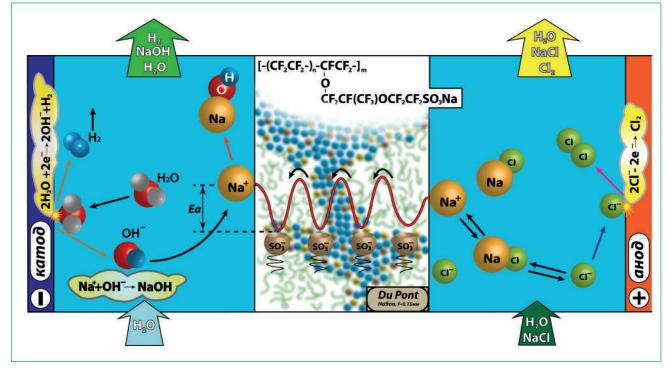
*Fig. 6.1.3.* Parameters of the process of charge transfer through the membrane is determined by speed of electromigration of cations in the polymer electrolyte. There is no pressure drop across the membrane. The process does not provide complete decomposition of the sodium chloride solution entering the anode chamber; it requires the introduction of distilled water into the cathode chamber.
