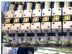
Chlorine capacity: 3 kg/h; Caustic soda productivity: 3.4 kg/h; Output of catholyte (18% aqueous NaOH solution): 19 l/h; Power consumption: 10 kW; Current strength — 2400 A; Voltage 4.4V; Overall dimensions (HxWxD): 1750x600x400 mm; Weight: 95 kg. Salt (sodium chloride) consumption: 5.4 kg/h; Salt consumption in solution (270–300 g/l): 18–20 l/h. **Provides disinfection of up to 72.000 m<sup>3</sup> of water per day.**
