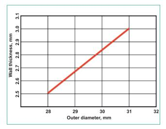
Fig. 6.1.6. Size ratio of ceramic diaphragms for MB-26 elements.
