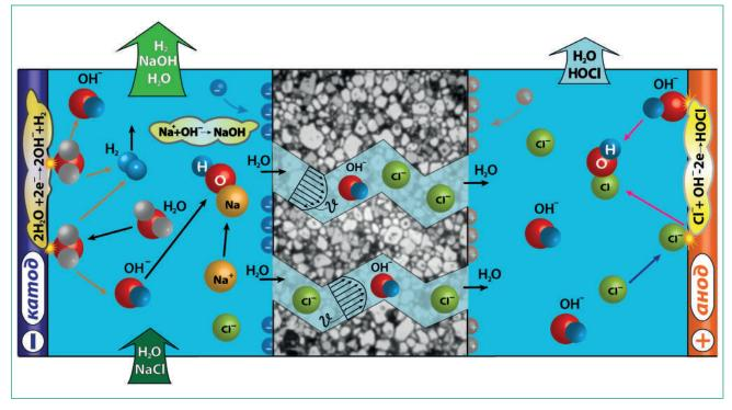
*Fig. 6.1.5.* A ceramic inactive diaphragm with pore sizes from 0.01 to  $0.1 \ \mu m$  turns into an anion-active MEMBRANE under the action of a superposition of the pressure field (from the cathode to the anode) and the electric field. The process ensures the production of a solution of caustic soda, hydrogen and hypochlorous acid from a sodium chloride solution with a concentration of up to 30%.
