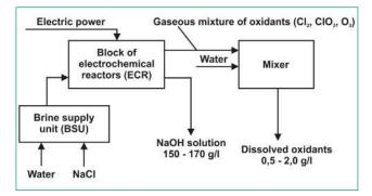
Fig. 5.5.1. Block diagram of AQUACHLOR device.
