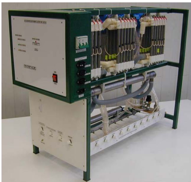
Figure 2. EMERALD device with productivity of 300 liters per hour. In the device is realized technological process TOPAZ of water treatment. Functional purpose: treatment of water from surface water sources at emergency situation. Power consumption – 800 Wt. Voltage at electrochemical reactor of the device is 24 V. It can be used as a part of mobile complex of water treatment or as a stationary device. Power supply from current source (rectifier) 220/30 V, or from car accumulator. Was produced in 2001 on demand of Department of Defense.
